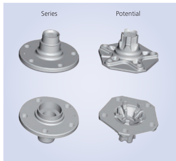
Figure 38: Wheel bearing – Comparison of the series part and the lightweight design proposal
