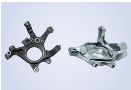
Figure 5: Car rear-axle wheel carrier – left: steel, right: next generation made of aluminium with reduced system weight
